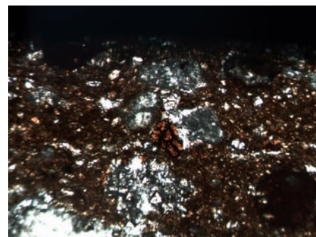
Fig. 17 Photomicrograph of sample 3 (xpl), showing a grain of iddingsite (center). Field of view 1.2 mm
